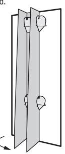
**2.** Fold the two stand braces downward until they lock with the stands.
